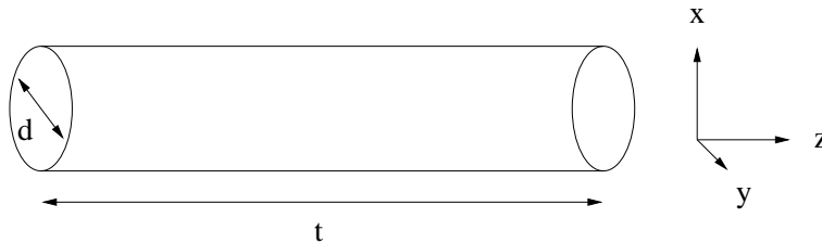
Figure 3.1: Circular cutoff waveguide with diameter d . The length is given by the thickness t of the plate and chosen at twice the diameter of the holes.
