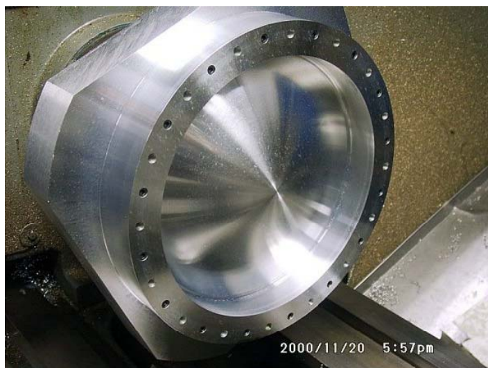
Figure 3.5.6: Liquid hydrogen absorber window built for safety tests in the US.
