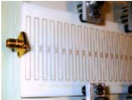
Figure 1: Chopper prototype, double 100 \Omega layout ( Z_0=50 \Omega )
