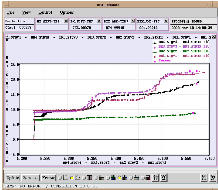
Figure 4: Intensity versus vertical tune for one turn injected and old working point optics. The drop of intensity when passing a resonance is clearly visible. The major sources of beam loss are the resonances 3Q_v = 16 and 2Q_v = 11 .
