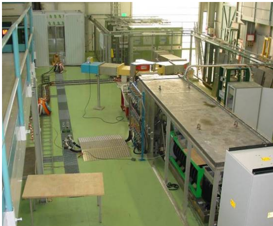
Figure 6: The Test Stand with klystron and modulator (right) and ion source cage (bottom).
