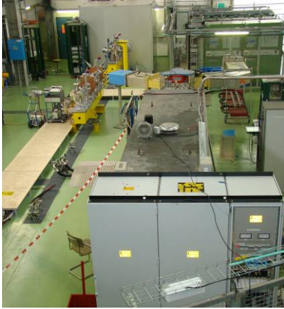
Figure 7: The Test Stand with klystron and modulator (right), ion source cage (top), chopper line (left).
