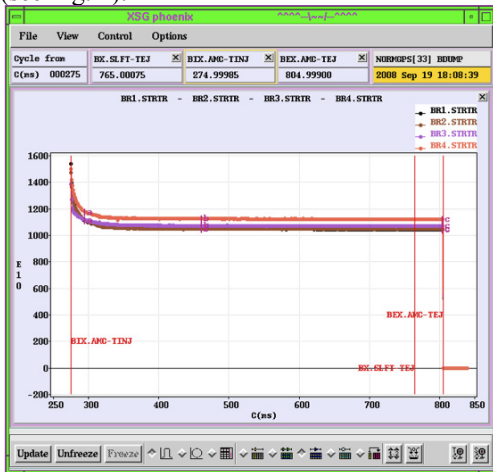
Figure 4: 2008 intensity record where almost 4300 \times 10^{10} protons were extracted for an ISOLDE beam and 13 injected turns.
