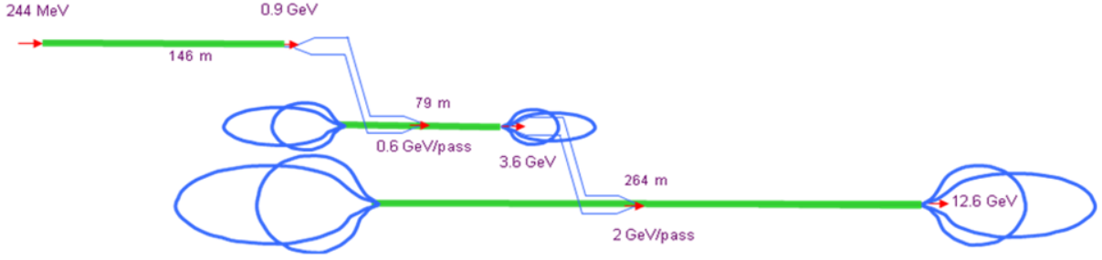
Figure 20: Layout of the accelerator complex. For compactness all components (the linac and the two RLAs) are stacked vertically; \mu^\pm beam transfer between the accelerator components is facilitated by the vertical double chicane (see text).
