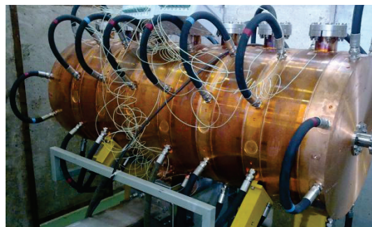
Figure 4: PIMS first cavity under high-power tests.
