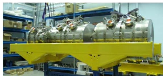
Figure 5: CCDTL module 2 during tests at Novosibirsk.
