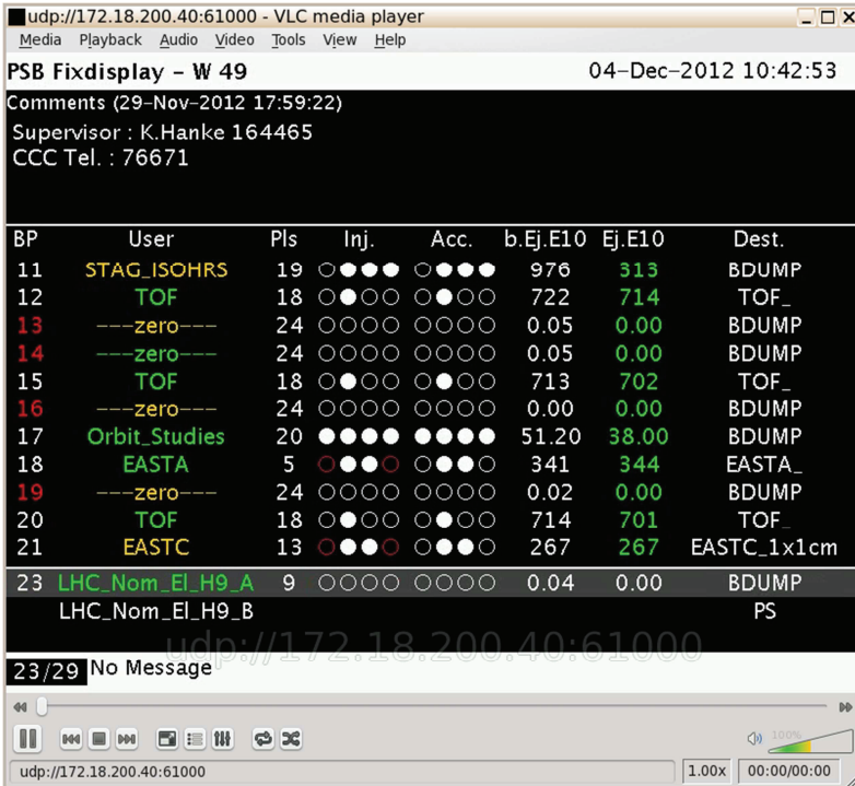
Fig. 16. Sequence of Booster cycles in a “supercycle”. The supercycle is composed of so-called basic periods of 1.2 s length. During each slot a beam for a given destination is injected, accelerated and extracted. Presently, most of the machine hardware and software can work in pulse-by-pulse modulation (ppm) mode, i.e. the single cycles are fully independent.
