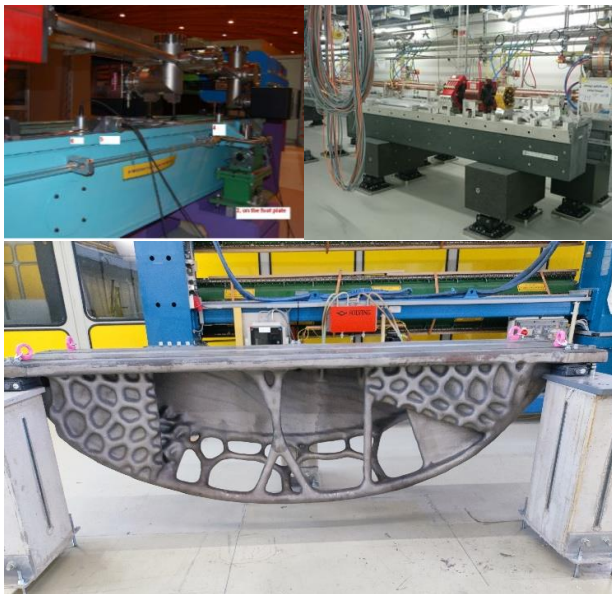
Fig. 5. Top left: steel girder for SLS, courtesy M. Wurm (PSI). Top right: granite girder for SwissFEL, courtesy J. Wickstroem (PSI). Bottom: cast girder for PETRA IV [9].
